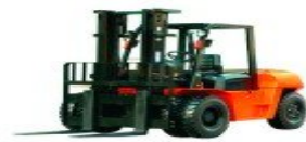
Medium Duty Diesel Capacity:5000-8000 Kg Lift Height :up to 6000 mm
