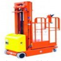
Electric Order Picker Capacity:350 Kg Lift Height :4500 mm
