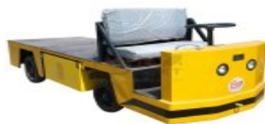
4 Wheel Platform Truck Capacity: 2000-4000 Kg
