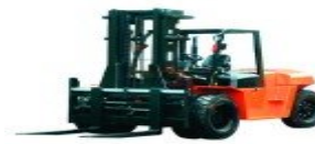
Heavy Duty Diesel Capacity:10000-16000 Kg Lift Height :up to 6000mm
